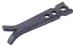
Erection Anchors are specifically designed for pitching and turning concrete units. They have specially designed nibs on the head of the anchor which prevent concrete from spalling when turning units. These are available in safe working loads from 1.4t to 22.0t.
