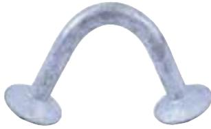
The Utility Anchor is designed for reinforced or unreinforced concrete units and is especially useful for cover slabs, pipes and culverts, or any application where the construction site can benefit from an approved and tested lifting anchor that can be used with a crane hook and no other special lifting device.
