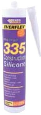
335 Construction Silicone is a low modulus reactive cure silicone sealant specially formulated as a cost-effective PVCu sealant, which also adheres to many common building substrates. It is fully tested to ISO 8339 and ISO 10590/10563.
