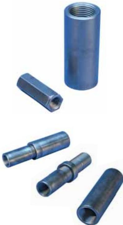
**Type A12N - LENTON standard coupler** - most widely used to splice bars. Designed to splice the same diameter bars where one bar can be rotated.
