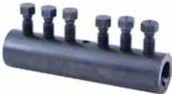
The MBT ET range of couplers provides a cost-effective method of joining reinforcing bars, particularly when the fixed bar is already in place and there is insufficient space for a hydraulic swaging press. This series of couplers is used to connect reinforcing bars of the same size.
