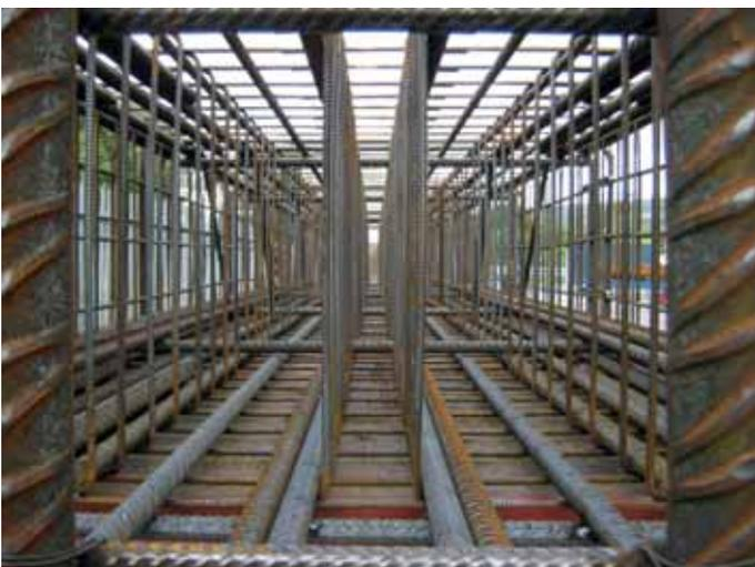
Prefabricated welded cages produced in accordance with BS 7123 & EN BS 17660.
