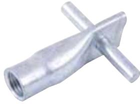
RFA-Tech Fixing Inserts with Cross Pin (Light Duty) provide a cost effective threaded fixing system in cast concrete with a strength of 30N/mm<sup>2</sup> and above, where either the unit or speed of installation required does not permit the use of a high yield reinforcement tail bar. They are effective for a single point fixing where no tolerance is required for attachment.
