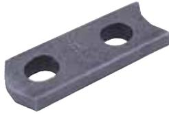
Two Hole Anchors are suitable for use where load distribution is not possible through the foot of a spread anchor and is done so by use of a reinforcement tail bar. They are particularly useful in thin wall panels and trusses, or where concrete strength is low. These are available in safe working loads from 0.7t to 22.0t.
