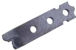
Universal Spread Anchors are for use in light duty applications and combine the benefits of Two Hole, Erection and Spread Anchors. They are available in 1.25t only, and use a former and ring clutch specific to this load group. They are suitable for small precast units or where a small recess is required.
