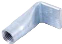
RFA-Tech Fixing Inserts with Right Angle provide a cost effective threaded fixing system in cast concrete with a strength of 30N/mm<sup>2</sup> and above, where either the unit or speed of installation required does not permit the use of a high yield reinforcement tail bar. They are effective for a single point fixing where no tolerance is required for attachment.
