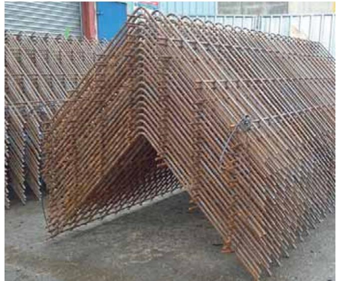
Most British standard shape codes can be accommodated but it may be necessary to manufacture them in sections for ease of transportation or to enable the shape to be completed.
