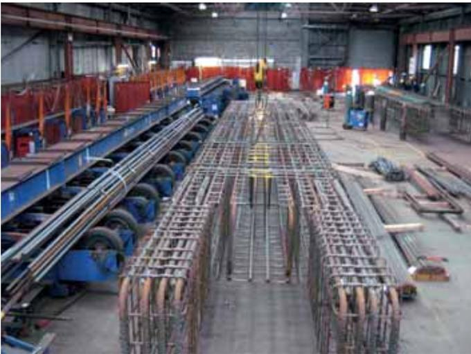
Cut and bent bar and prefabricated units are produced in accordance with BS 8666:2005
