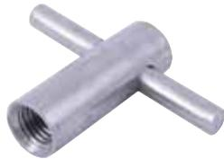
RFA-Tech Fixing Inserts with Cross Pin (Heavy Duty) provide a cost effective threaded fixing system in cast concrete with a strength of 30N/mm<sup>2</sup> and above, where either the unit or speed of installation required does not permit the use of a high yield reinforcement tail bar. They are effective for a single point fixing where no tolerance is required for attachment.
